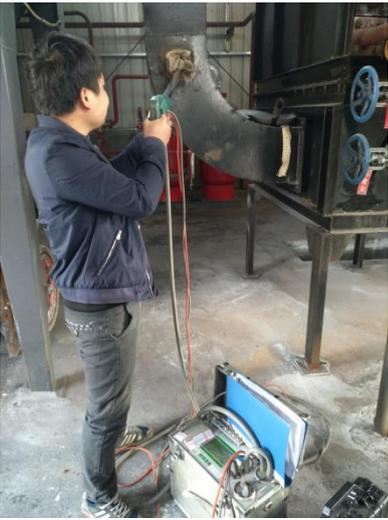
A photograph showing organized gas sampling. A person is using a sampling device to collect gas from a large, dark, cylindrical machine. A laptop computer is open on the ground, displaying data from the sampling process.           |
